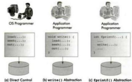
Let us see how disk output operations can be represented at different levels of abstraction. The device is controlled with software operations for copying a block of information from the computer's main memory into the device's buffer memory.
