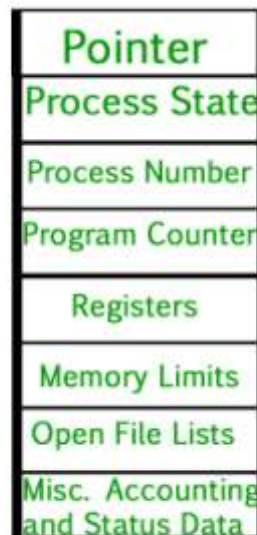
Process Control Block
