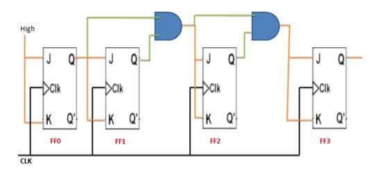
Fig: 4 bit Synchronous binary counter
